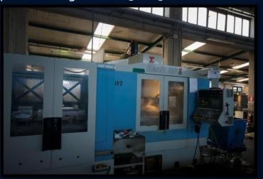
2 Vertical Work centers AWEA BM 1200 1200x600x600 – (Equipped with Fanuc oi-MD)
